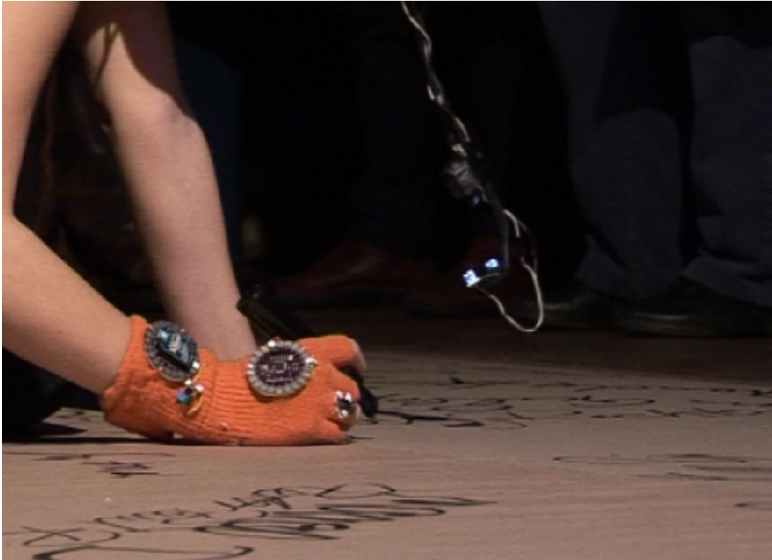
Figure 32: Glove with accelerometer, Arduino LilyPad, xBee and a switch for triggering the new name on the projection.
