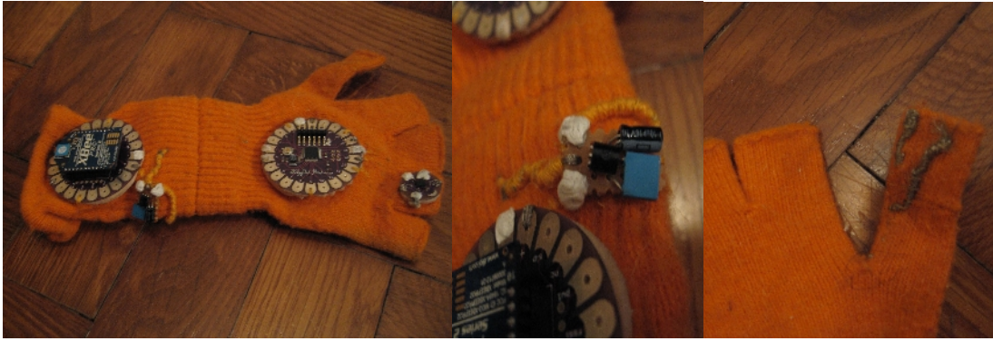
Figure 33: On the left, the glove with LilyPad and xBee, middle, close up of the voltage regulator, and right, close up of the switch.
